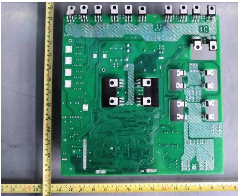
Power board view (Soldered side)
